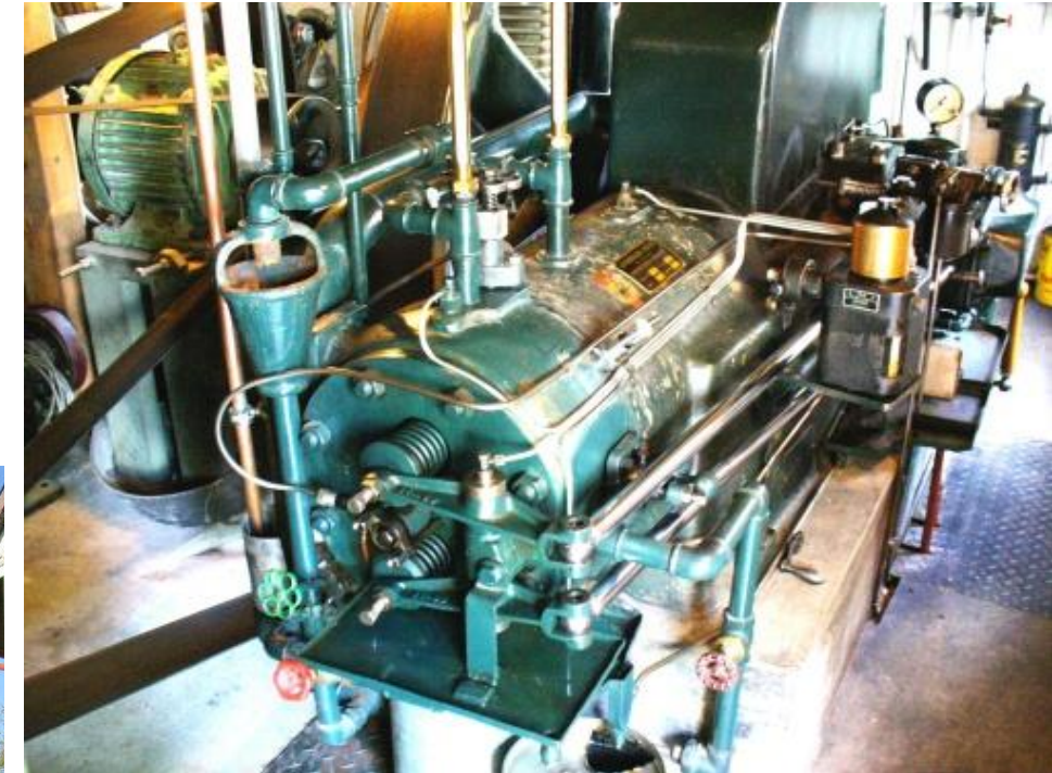
60 year old Ossberg pressure turbine – Moulin Mellert Freiamt (15 KW) Source: Mellert Mühle
